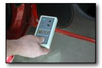
If the system is already up and running you can use the Test CD on track 3 to allow the instrument to "listen" for the pulse signals. Position it near the speaker and watch for 3 green pulses followed by 1 red pulse.
