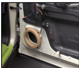
This process can also be used for creating perfect fit door speaker adapters
